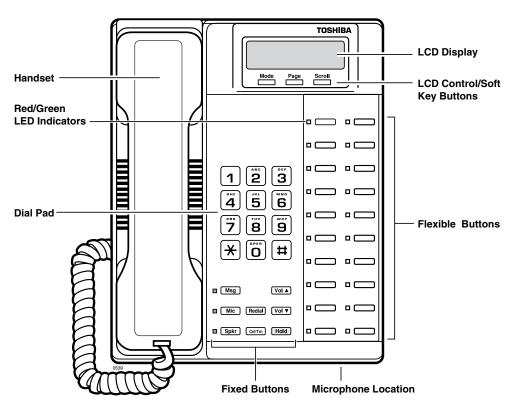
Figure 1 20-button Digital Speakerphone with LCD
